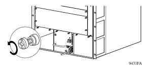
5. Loosen the retaining screws on the power supply.
